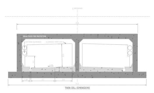
Figure 6 Typical Cross-Section of Twin Cell Tunnel - West Apron Vehicle Underpass
