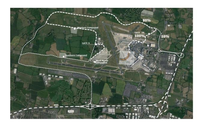
Figure 14 Site Access & Haul Routes Phase 3 (Post closure of Runway 16/34)
