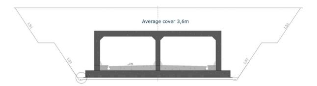
Figure 8 Typical Underpass Cross-Section including benched excavation slopes
