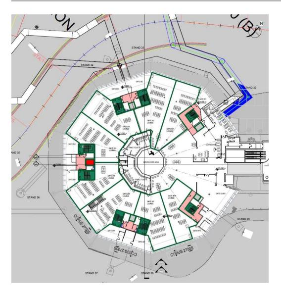
A new partition creating an airlock will be required between the entrance/ exits of Fixed Links A and B to ensure full segregation of departing and arriving passengers. Fixed Link C has been positioned to join the departures level where it has the least impact on the existing food and beverage concession. Due to the retained stand arrangement to the South, no changes are required to the fixed links and gate lounges serving these stands.
