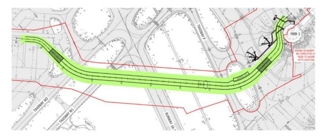
Figure 5 Proposed West Apron Vehicle Underpass Alignment
