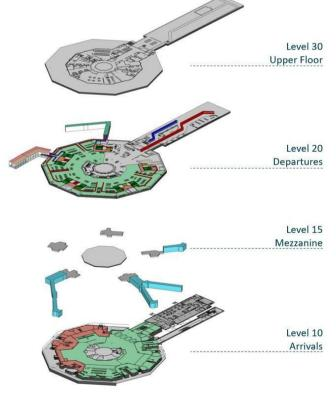
The Pier 3 decagon comprises of four levels including Level 30 office accommodation, Level 20 departure gates with open lounges, Level 15 mezzanine providing access to the fixed links and nodes and Level 10 arrivals immigration hall.
