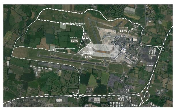
Figure 13 Site Access & Haul Routes Phase 2 (During closure of Runway 16/34)
